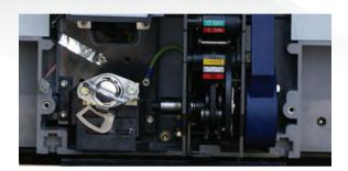
Ready-to-fit interlocking devices such as Castell, Ronis, Profalux and Fortress, for installation between separate circuit breakers, available in kit form. This valuable safe guard ensures that a circuit breaker cannot be closed unless the dedicated key has been inserted and secured within the lock.
