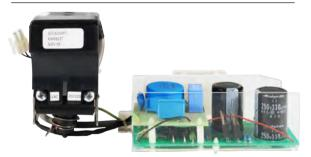
Instantaneously releases the circuit breaker trip mechanism when the supply voltage dip below the pre-set value. Simple to install, these devices have the same easy-fit features as previously described. Note: This is a 'no-volt/no-close device. The circuit breaker cannot be closed (manually or electrically) unless the undervoltage release coil is energized.
